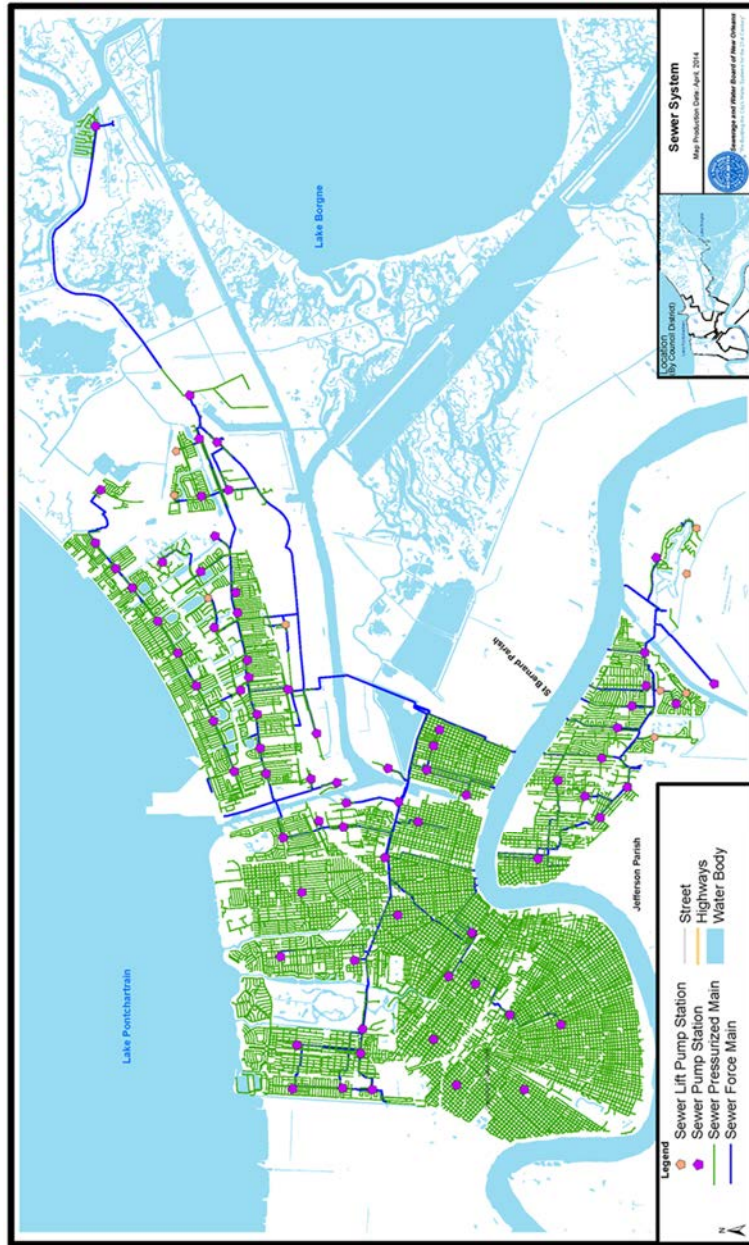
Figure 4-1 Overview of the SWBNO Sewerage System
